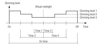
The different predefined chronoSTEP scenes can be chosen via ON/OFF cycles of the mains supply voltage (programming mode 2).
