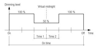
Time 1 and Time 2 can be set via ON/OFF cycles of the mains supply voltage (programming mode 1).
