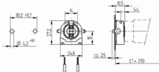
L1+21.0: Recommended dimension - The distance between the cut-outs and the tolerance should be governed by the dimensions of the respective lamps and luminaires.
